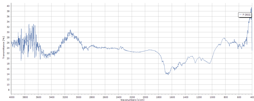
Figure 1(a): Powdered fish scales FTIR spectra.
