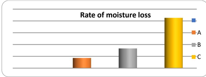
Key: A - Open Sun Drying; B - Solar Drier with Single Cover; C - Solar Drier with Double Cover
