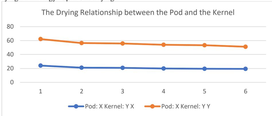
Figure 7: Drying Relationship between the Pod and the Kernel in Open Sun Drying.
