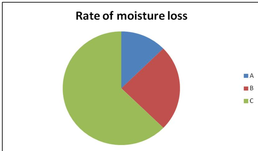
Key: A - Open Sun Drying; B - Solar Drier with Single Cover; C - Solar Drier with Double Cover
