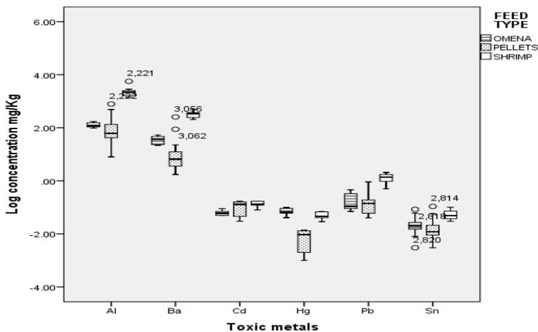
Figure 4: Box Plots showing potential toxic elements (PTEs) concentration in mg/kg for *in-situ* based feeds and formulated feed pellets (mg/kg; wet weight).
