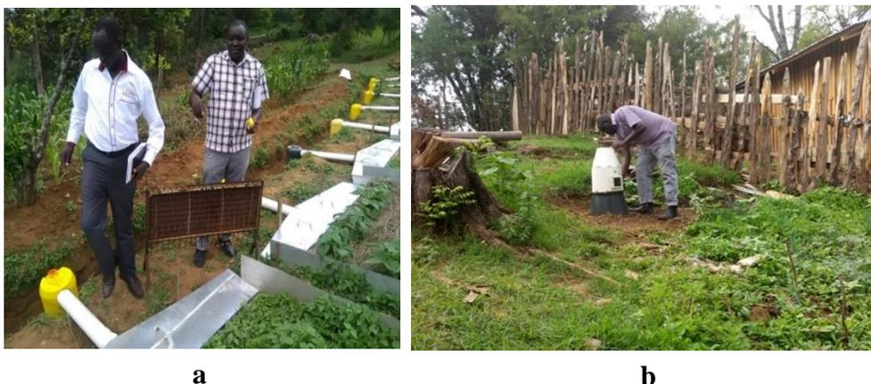
Figure 6: Run-off collection (a) and rain gauge installation (b).
